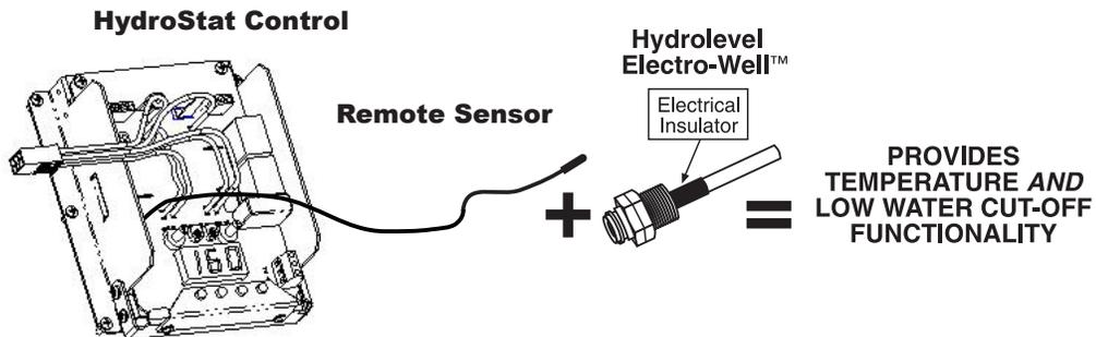
**Important:** The PWXL Boiler is equipped with a HydroStat Electro-Well. Do not replace the Electro-Well with a standard immersion well or the low water cut-off function will be disabled.
