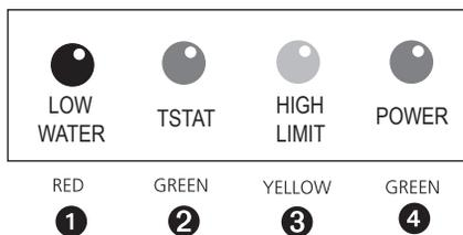
**3 HIGH LIMIT** Illuminates when the boiler water temperature reaches the high limit setting. It will remain lit until the water temperature falls below the high limit setting less the differential setting. The HydroStat control will prevent burner operation while this LED is on.
